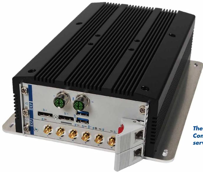
***The ELOS rugged embedded system platform is based on CompactPCI Serial. With its modular approach, it can serve a variety of applications.***
