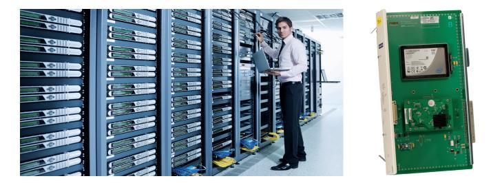
This 6U "VME-like" disk module uses the latest drive technology in a backwards compatible form, fit and functional replacement module for use in optical switching equipment for the telecommunications industry. Variations of this product can be used in many applications requiring custom storage solutions.
