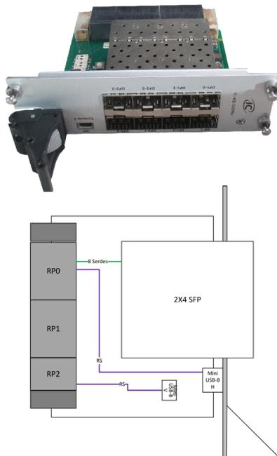
The **ComEth4590a** also supports VPX System Management in compliance with VITA 46.11 and based on the Intelligent Platform Management Interface (IPMI v1.5) for sensor management (temperature, voltage, current), inventory management, system configuration, recovery and diagnostic management.
