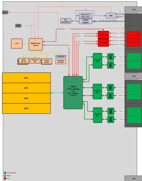
The **ComEth4341e** is compliant with the VITA 65.0 Slot Profile SLT6-SWH-4F24T.
