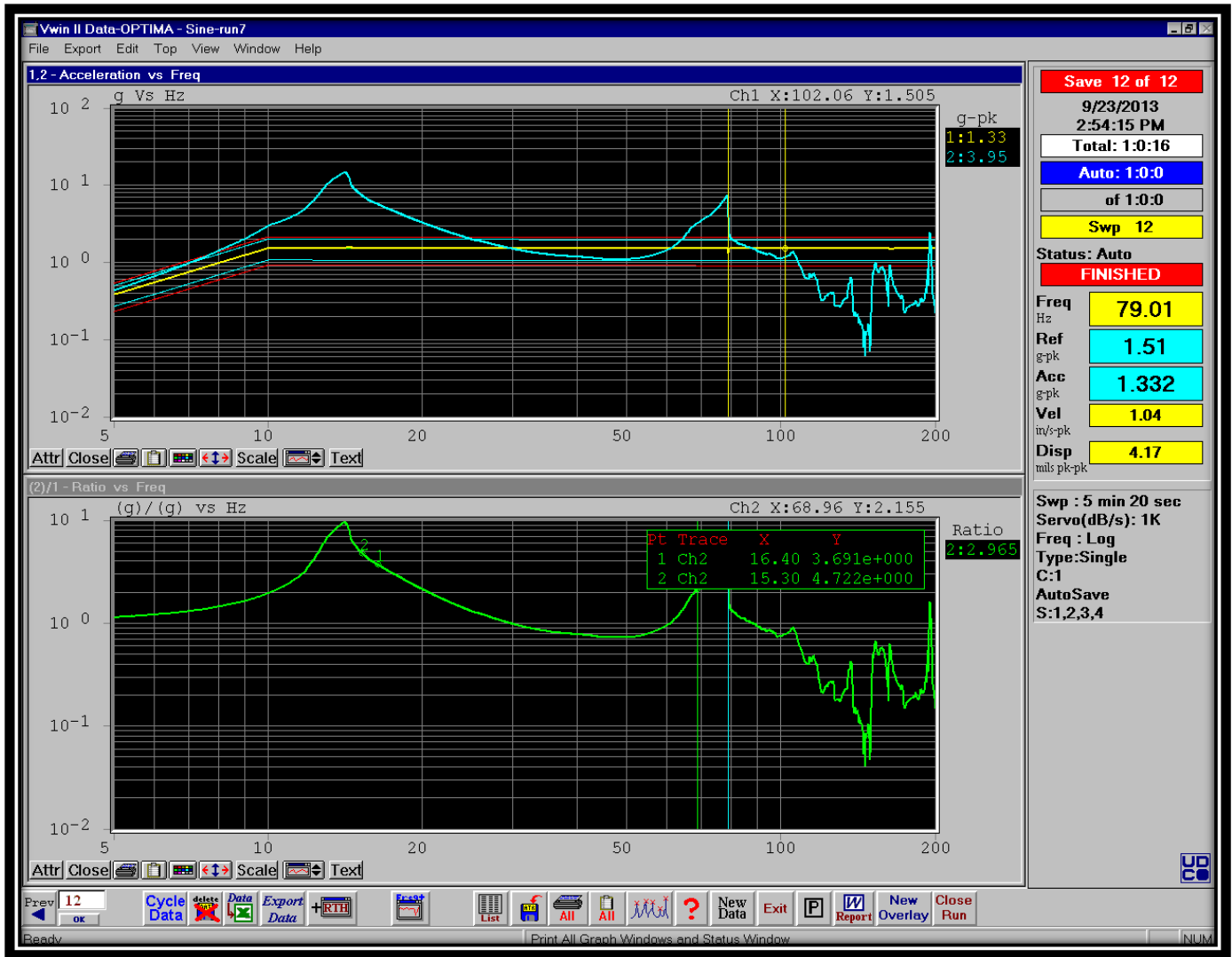
Figure 4: AREMA profile – Sinusoidal vibration – Longitudinal Direction
