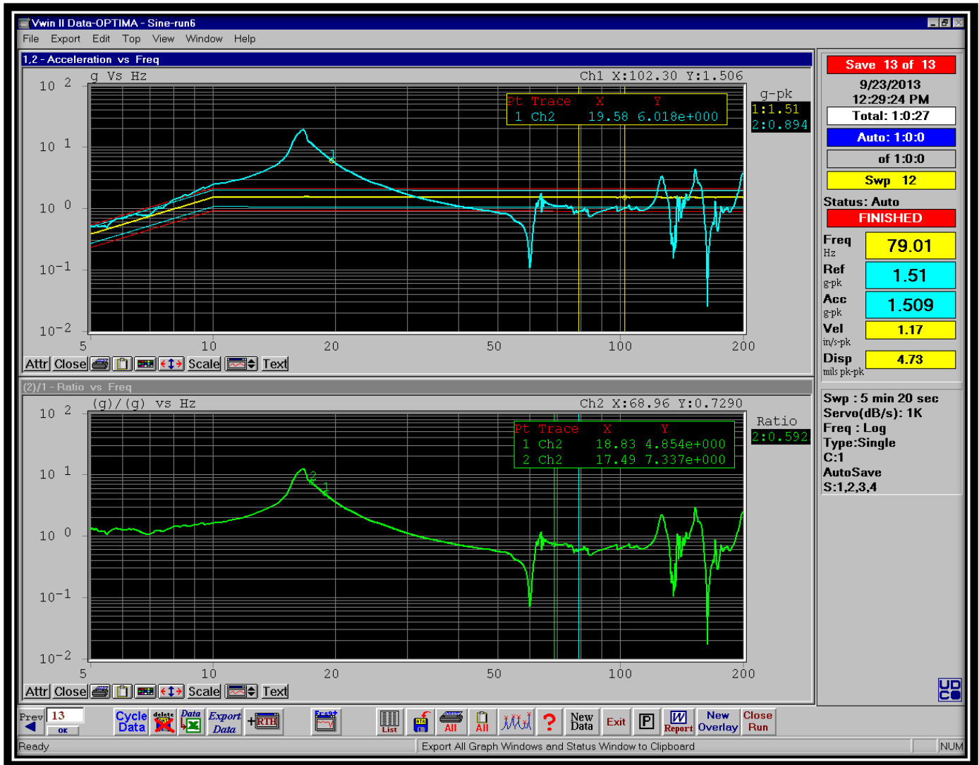
Figure 5: AREMA profile – Sinusoidal vibration – Transverse Direction
