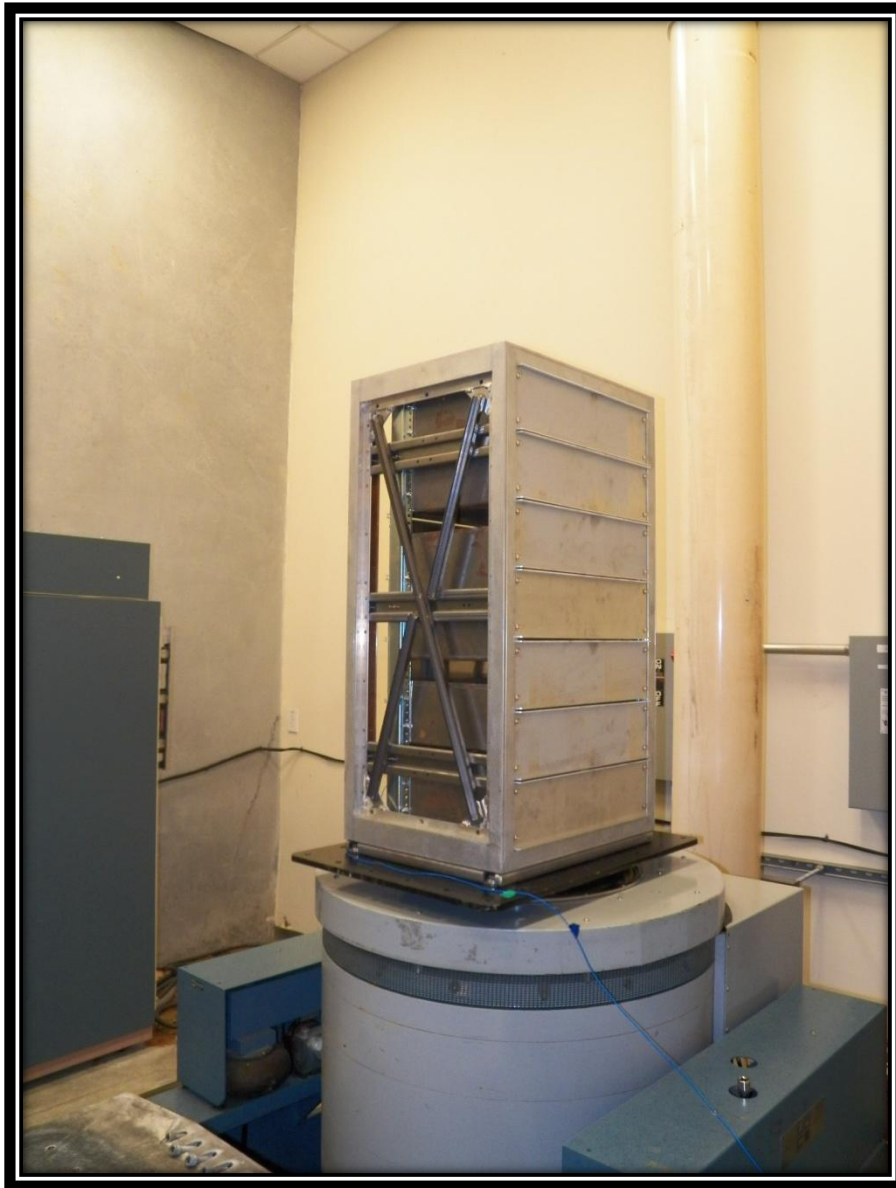
Figure 3: View of the test setup – Vertical Direction
