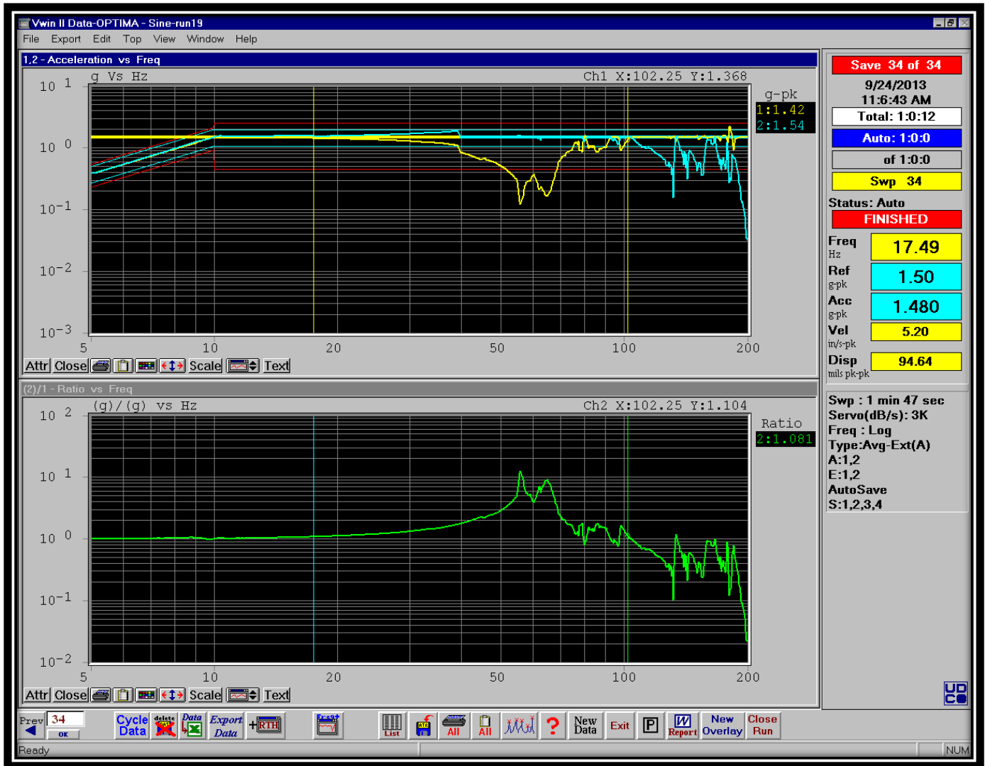
Figure 6: AREMA profile – Sinusoidal vibration – Vertical Direction
