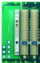
9 – DIN 41612 Type M, 4-8 slot 3U: Lower position 6U: Upper und lower position
