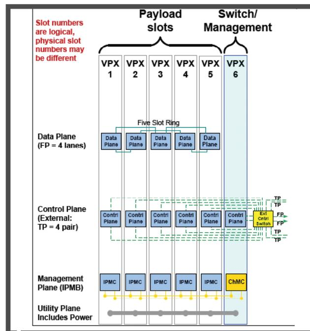
The backplane configuration examples show the connectivity across the backplane for various planes. This includes the routing topology across the data plane and the connections across the expansion, control, management and utility planes. They also provide an illustration of the slot types, whether payload, switch or legacy bus slots.
