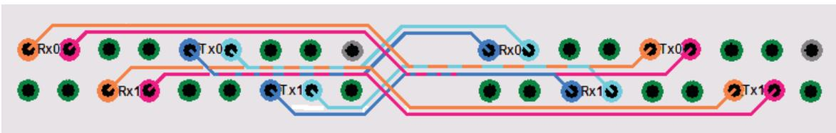
**Ultra-thin Pipe:** A channel that is comprised of one link (1 Tx pair + 1 Rx pair) is now being referred to as an ultra-thin pipe or by use of the x1 nomenclature. 10GBase-KR, 10GBase-KX, PCIe-x1, sRIO-x1, Infiniband-x1a
