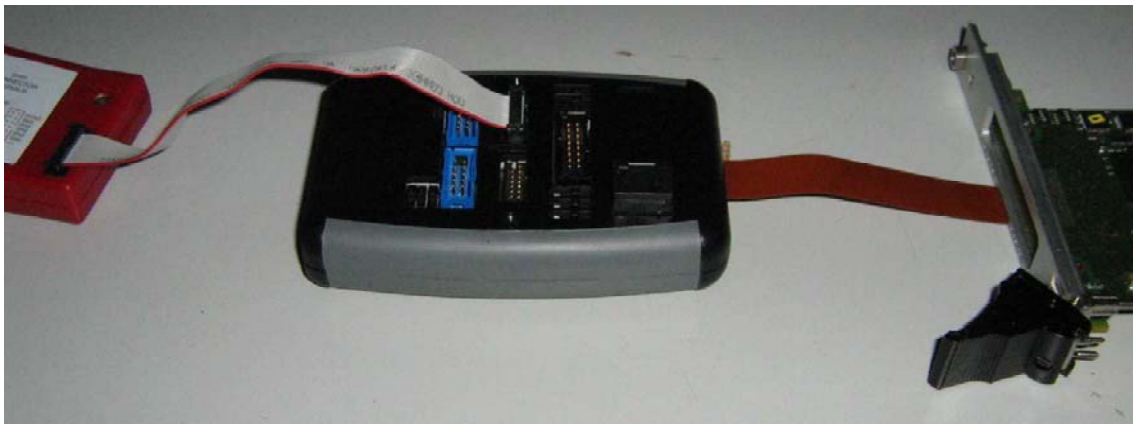
Figure 9 Typical Engineering Kit Pods showing connection to FPGA carrier via JTAG
