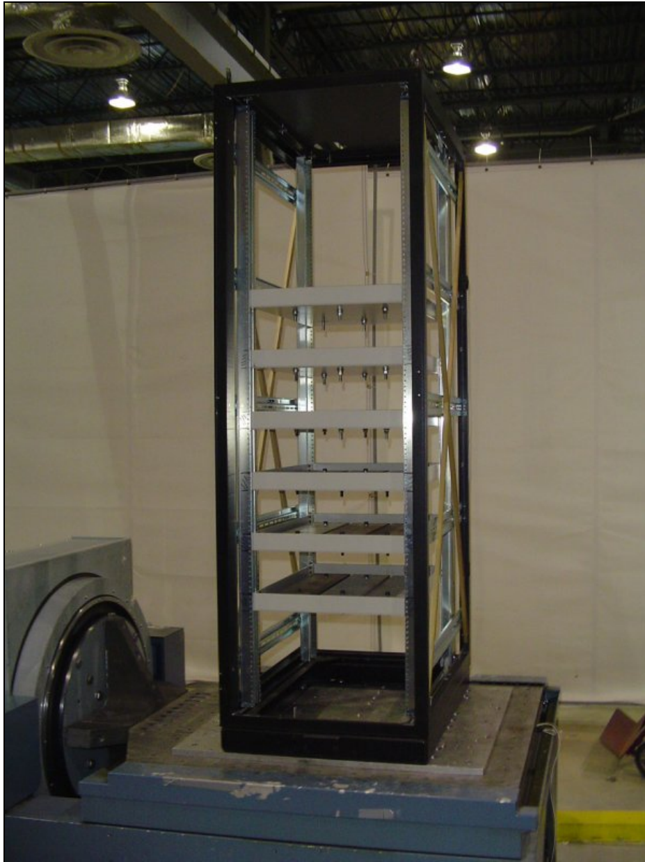
Photograph 6. Shock, Transverse Axis Test Setup
