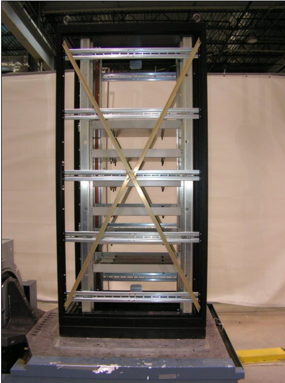
Photograph 2. Vibration, Longitudinal Axis Test Setup
