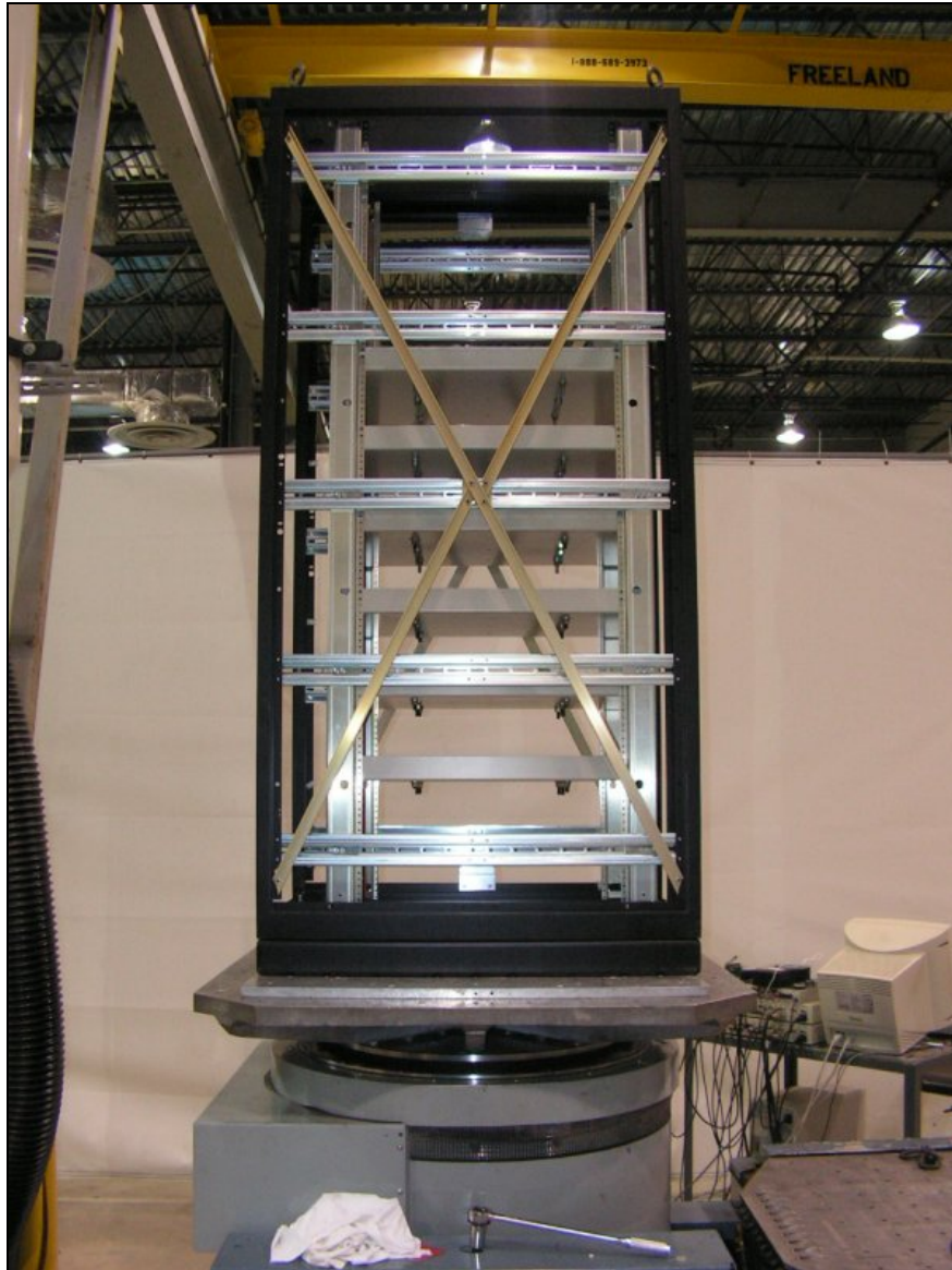
Photograph 1. Vibration, Vertical Axis Test Setup
