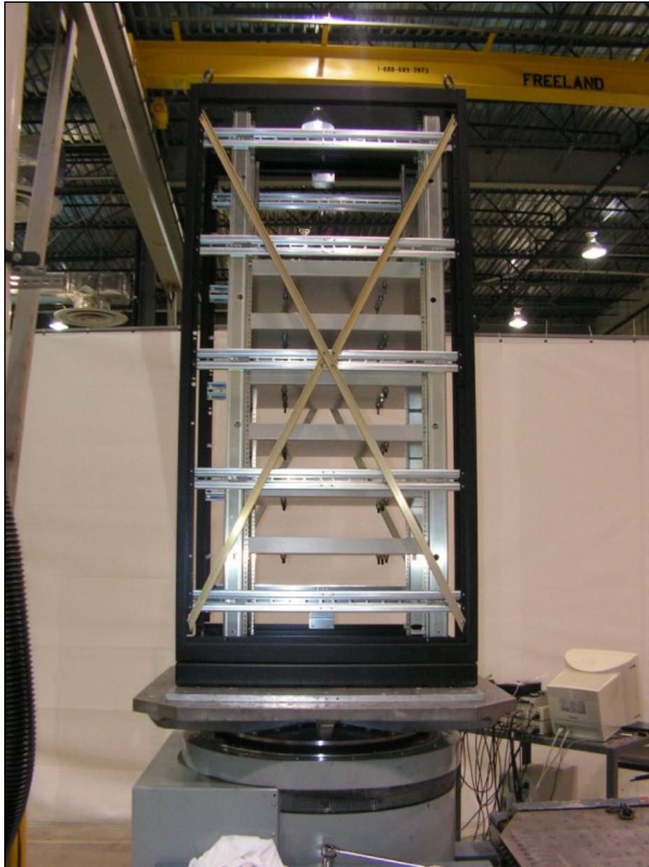
Photograph 4. Shock, Vertical Axis Test Setup
