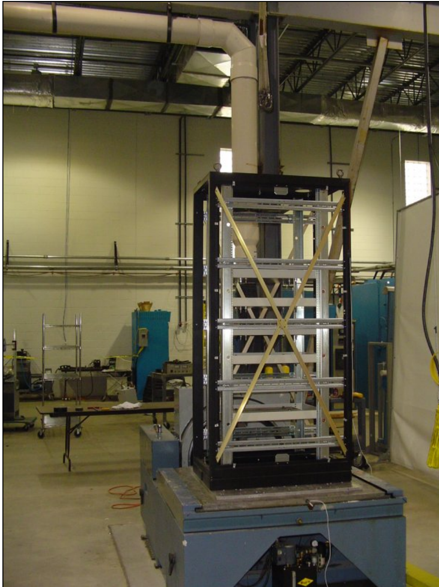
Photograph 3. Vibration, Transverse Axis Test Setup
