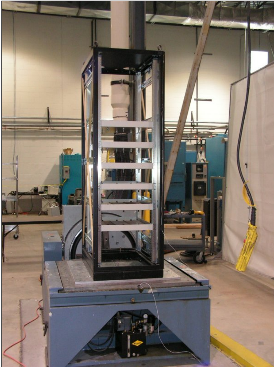
Photograph 5. Shock, Longitudinal Axis Test Setup
