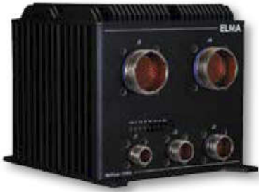
Figure 3 The NetSys-5303 features both mechanical and functional modular concepts for scalability.
