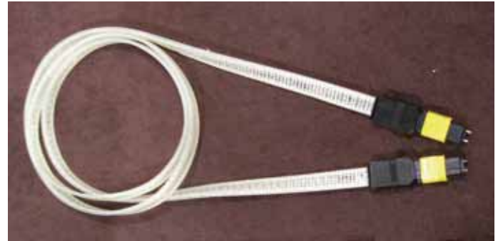
Figure 1: A 12 optical fiber ribbon terminated to an MT ferrule.
