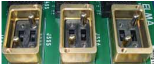
Figure 2: Top: Hybrid VME/VPX backplane with VITA 66.1 optical connectors and VITA 67.2 coaxial copper connectors and standard VITA 46 MultiGig connectors in positions J0-J4. Bottom: Optical ferrules close up.
