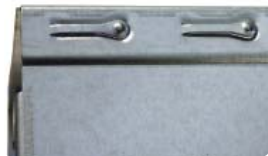
Figure 3: Stamped or formed EMC gasketing can be applied directly into the sheet metal or aluminum. Strips offer flexibility of location, while forming can mean less individual parts and assembly.
