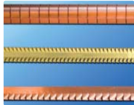
Figure 3: Stamped or formed EMC gasketing can be applied directly into the sheet metal or aluminum. Strips offer flexibility of location, while forming can mean less individual parts and assembly.
